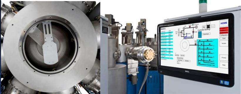
*Example of FLEX3008- Six (6) PECVD process zones with a central robotic module for vertical upwards deposition up to 8" (3008) round wafers and 400°C substrate heating capability*
