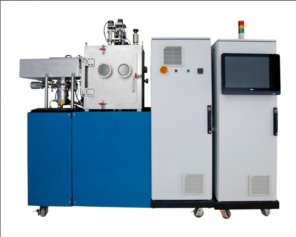
FLEX2000- stand alone multi process chamber tool with deposition up to 2" (2002), 4" (2004) and 8" (2008) round wafers. Multiple and co-depositions up to six sources using either sputtering or thermal evaporation , substrate rotation and 400°C substrate temperature standard. State of the art thin film process recipe for various thin films.
