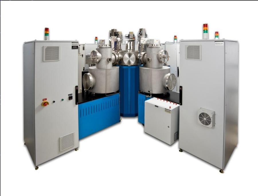
Example of FLEX3004- four (4) PECVD process zones, two (2) multi-source magnetron sputtering zones and a hot wire CVD (HWCVD) zone with a central robotic module for vertical upwards deposition up to 4" (3004) round wafers up to 400°C substrate heating capability
