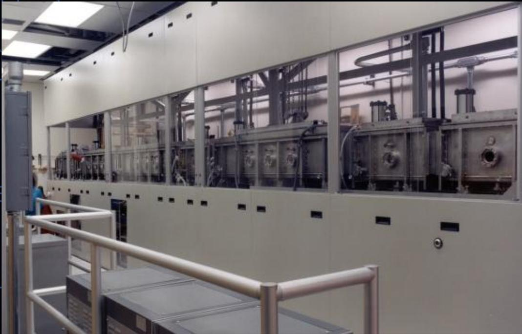
FLEX5000- Inline multi process and multi chambers prototyping production tool, with deposition up to 20" square substrates. Processes include PECVD, HWCVD, ICP and Sputtering. State of the art thin film process recipe for various thin films and devices
