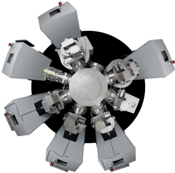
FLEX3000- Multi process and multi chambers tool, up to eight (8) process zones (Cluster Tool) with a central robotic module with deposition up to 4" (3004) and 8" (3008) round wafers. Processes include PECVD, HWCVD, ICP and Sputtering. State of the art thin film process recipe for various thin films and devices
